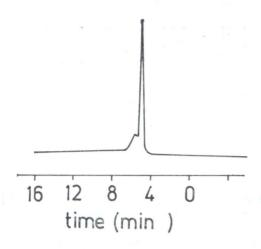
Fig. 2. HPLC of STFc on a 0.45 × 24 cm column of octadecyl silane Chromatography was performed at a flow rate of 0.62 ml/min under 70 BAR. Meth-
